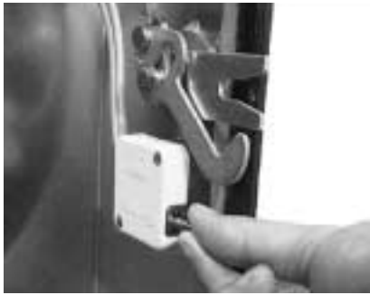
Fig. 20 Pulling of service switch
