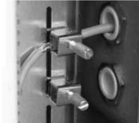
Fig. 7 External connection to the I/O terminals
